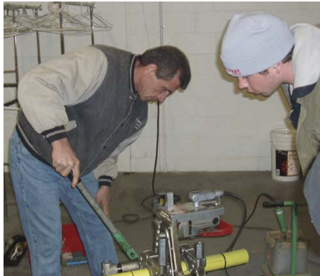
Nick Furness proud of his butt fusion joint with apprentice Rynell Jackson and journeyman Joe Cass watching
