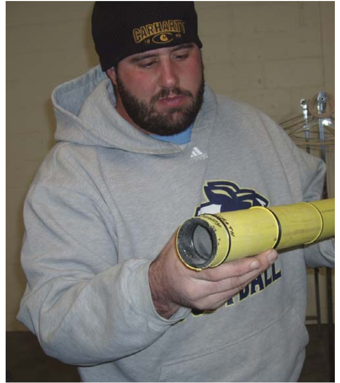
Mike Piccirillo inspecting his fusion butt joint on 2-inch pipe
